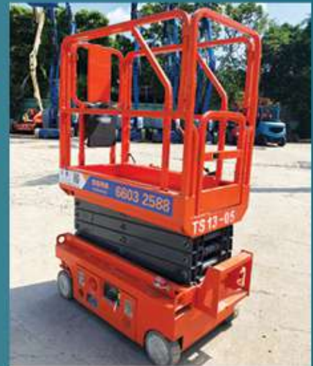
Brand: Dingli Model: JCPT0607DCS Type: Electric Scissor Lift Platform Height: 3.9m Year: 2016 - 2018
