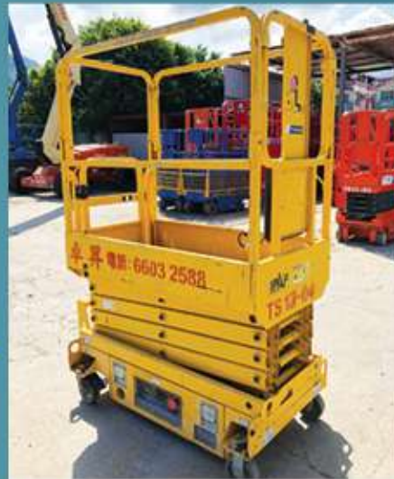
Brand: Dingli Model: JCPT0607 Type: Electric Scissor Lift Platform Height: 3.9m Year: 2015 - 2016
