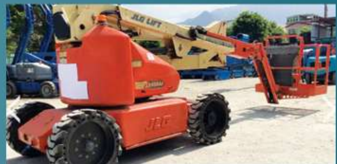
Brand: JLG | Model: E450AJ | Type: Electric Boom Lift Platform Height: 45ft. | Year: 2007
