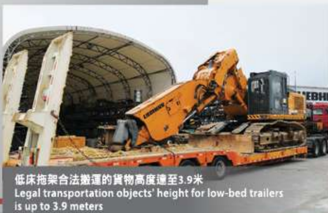
拖架 最高載重150噸 (內運300噸) TRAILERS MAXIMUM 150 TONS ON ROAD (300 TONS ON SITE)
