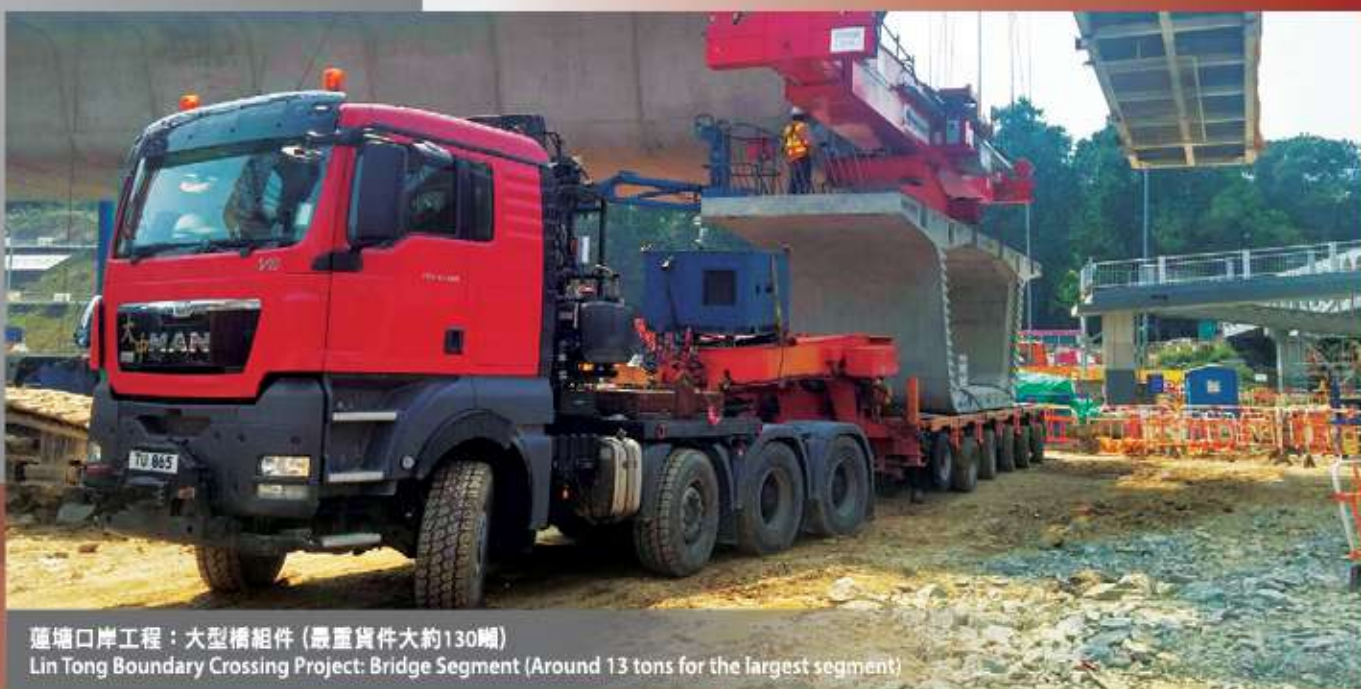
低床拖架合法搬運的貨物高度達至3.9米 Legal transportation objects' height for low-bed trailers is up to 3.9 meters
