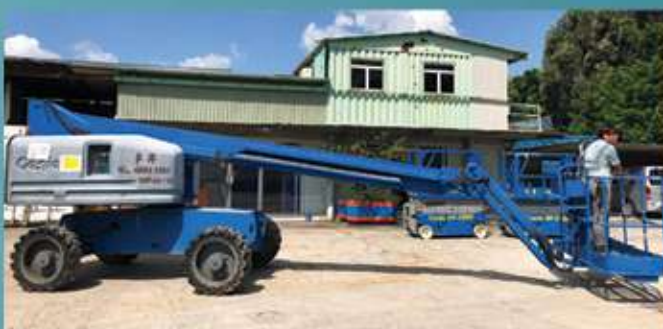
Brand: Genie | Model: S45 | Type: Diesel Boom Lift Platform Height: 45ft. | Year: 1999
